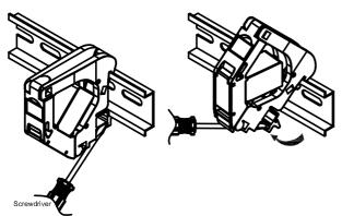
Insert a screwdriver into the opening at the bottom of the module and use it as a lever to pull out the module.
