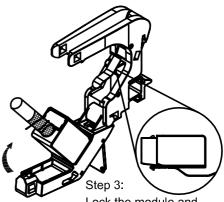
Lock the module and make sure the grounding spring contacts the jack to ensure grounding connection.
