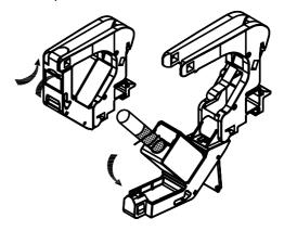
Use screwdrivers or fingers to open the poles at the top of the module.
