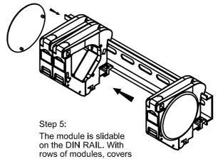
on the DIN RAIL. With rows of modules, covers are only needed for the right and left ends of the row.
