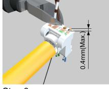
Step 3: Trim excess wires. The tips of the wires should protrude no more than 0.4mm.
