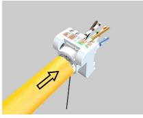
Step 2: Put wires through wire management and arrange in accordance with wiring color code (T568A/B).
