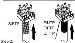
Insert the wires into the cap through the holes.
