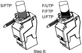
Fix the cable tie to the shielding lug.
