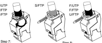
The drain wire should be wrapped around the strain relief as shown to ensure 360° shielded.
