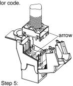
Put the cap on the IDC tower. The arrows on the jack and the cap should face the same direction. Put the cap into postion.
