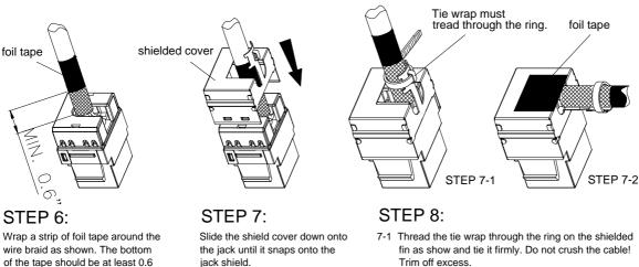
Johannesfredsvägen12 SE-168 69 Bromma Sweden 7-2 Bend the cable perpendicular to the jack and secure the foil tape over the opening in the cover as shown.
