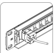
b. With the bottom latch engaged to the patch panel, rotate the jack upward until the flexing side of the keystone latch engages with the patch panel. There should be a slight clicking sound as the latch engages.
