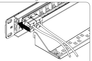
Align the tongue of the wire minder with the corresponding groove on the patch panel and insert it into the groove.
