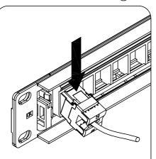
a. Insert the jack into its opening in the patch panel at an angle with the non-flexing side of the keystone latch facing down.
